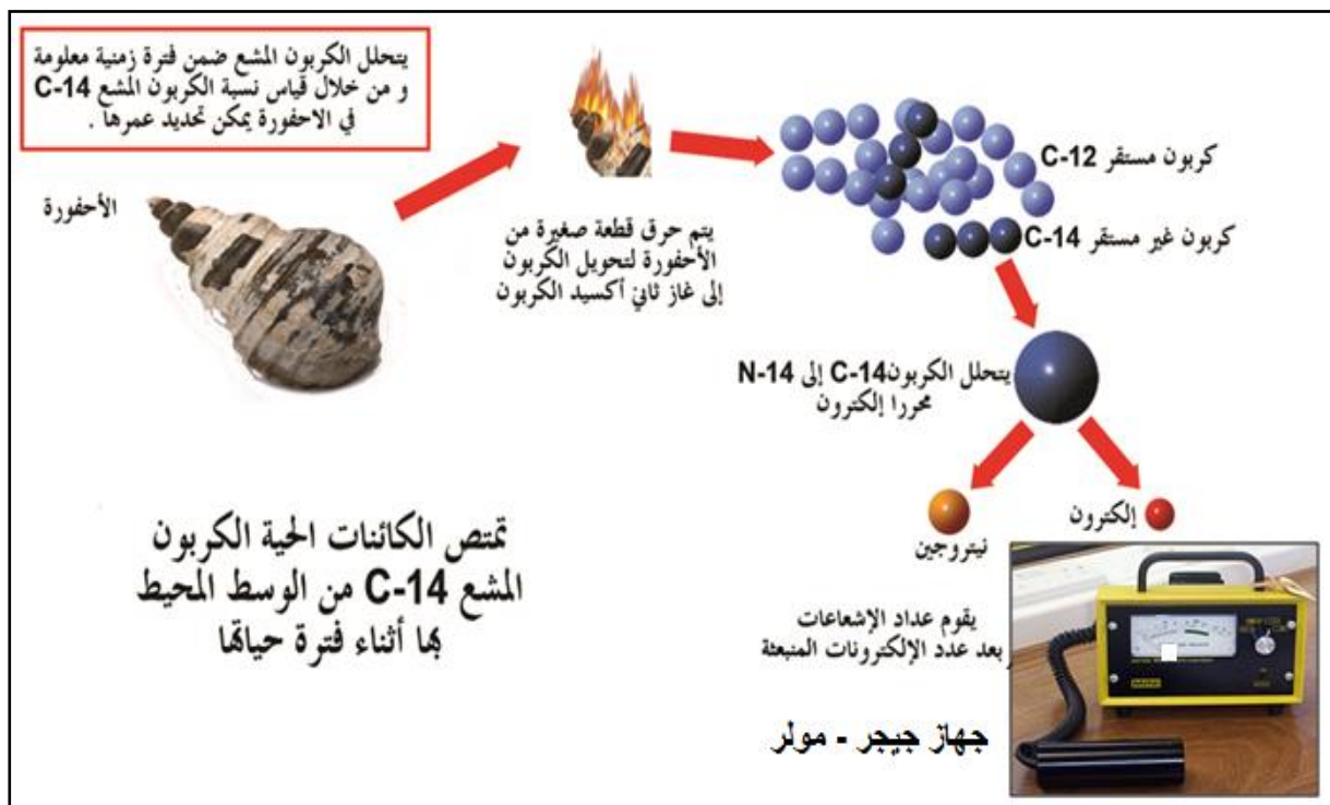
Figure No.: Steps followed in determining the age of an antiquity using the Geiger-Muller device
